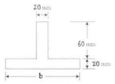
b) If the moment of inertia of the shaded area(25 cm<sup>2</sup>) shown in fig. about 1-1 axis is 7400 cm<sup>4</sup> then determine the moment of inertia of area about 2-2 axis.
